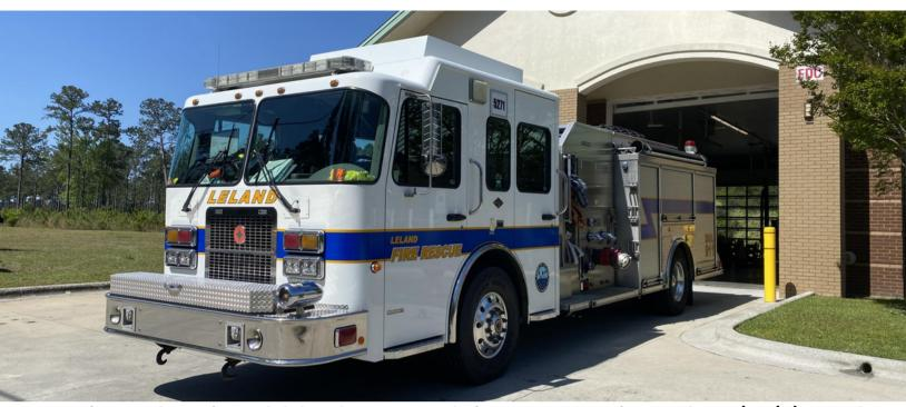
Engine 5371 is a 2007 Spartan Crimson. Engine 5371 holds 750 gallons of water and has a 1500 gpm pump. It is housed at Station 53.
