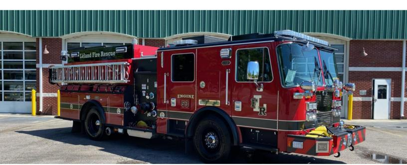
Engine 5271 is a 2022 KME Custom Pumper. Engine 5271 holds 750 gallons of water and has a 1500 gpm pump. It is housed at Station 52.
