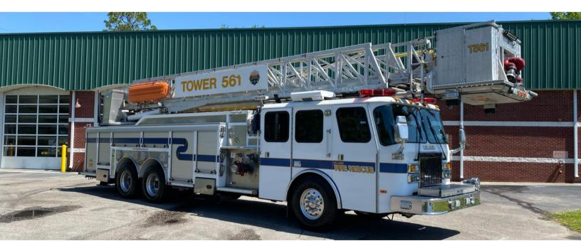
Truck 5361 is a 2001 E-One Tower. It is a rear-mount platform with 300 gallons of water and a 2000 gpm pump. It is housed at Station 53.
