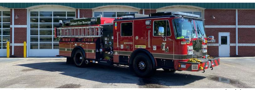
Engine 5171 is a 2022 KME Custom Pumper. Engine 5171 holds 750 gallons of water and has a 1500 gpm pump. It is housed at Station 51.
