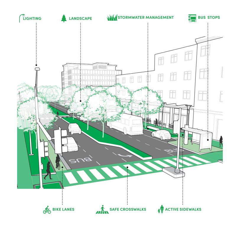
**Figure 4:** Example of typical principles and components considered in complete streets with the ultimate goal of safety, mobility and accessibility for all users including pedestrians, bicyclists, motorists, and transit riders of all ages and abilities. These components will look different depending on their context, whether that is rural, urban, or suburban.
