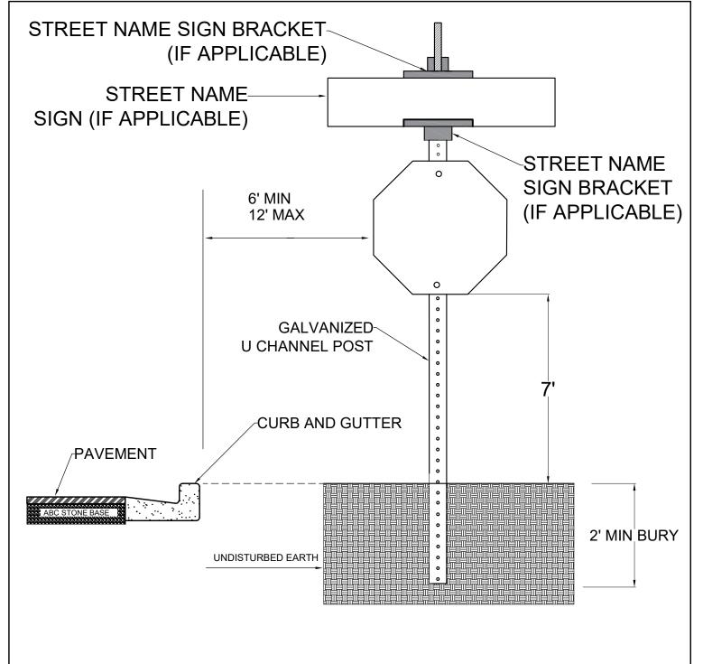
ALL SIGNS MUST MEET THE MUTCD REQUIREMENTS FOR SIZE, HEIGHT ABOVE THE GROUND, AND REFLECTIVITY.
