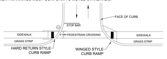
DETAIL SHOWING TYPICAL LOCATION OF SIDEWALK ACCESS RAMPS PEDESTRIAN CROSSWALKS, STOP SIGN, AND STOP BARS FOR "T" TYPE INTERSECTION. SIDEWALK ON ONE SIDE OF THE THRU STREET. STOP BAR SHALL BE IN FRONT OF CROSSWALK.
