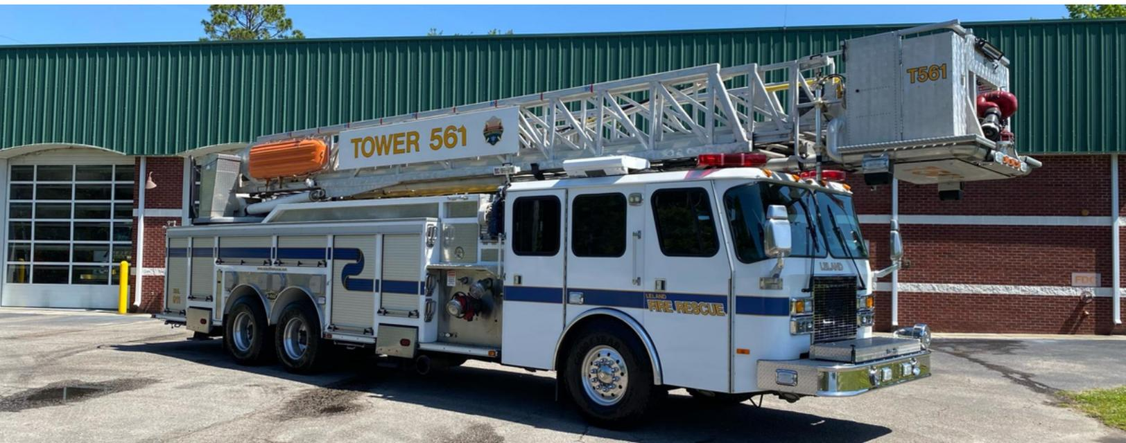
Truck 5361 is a 2001 E-One Tower. It is a rear-mount platform with 300 gallons of water and a 2000 gpm pump. It is housed at Station 53.
