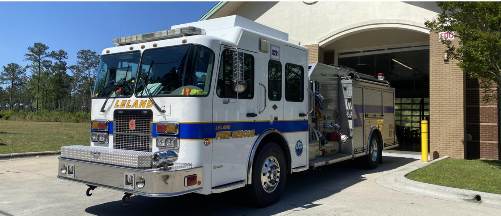
Engine 5371 is a 2007 Spartan Crimson. Engine 5371 holds 750 gallons of water and has a 1500 gpm pump. It is housed at Station 53.
