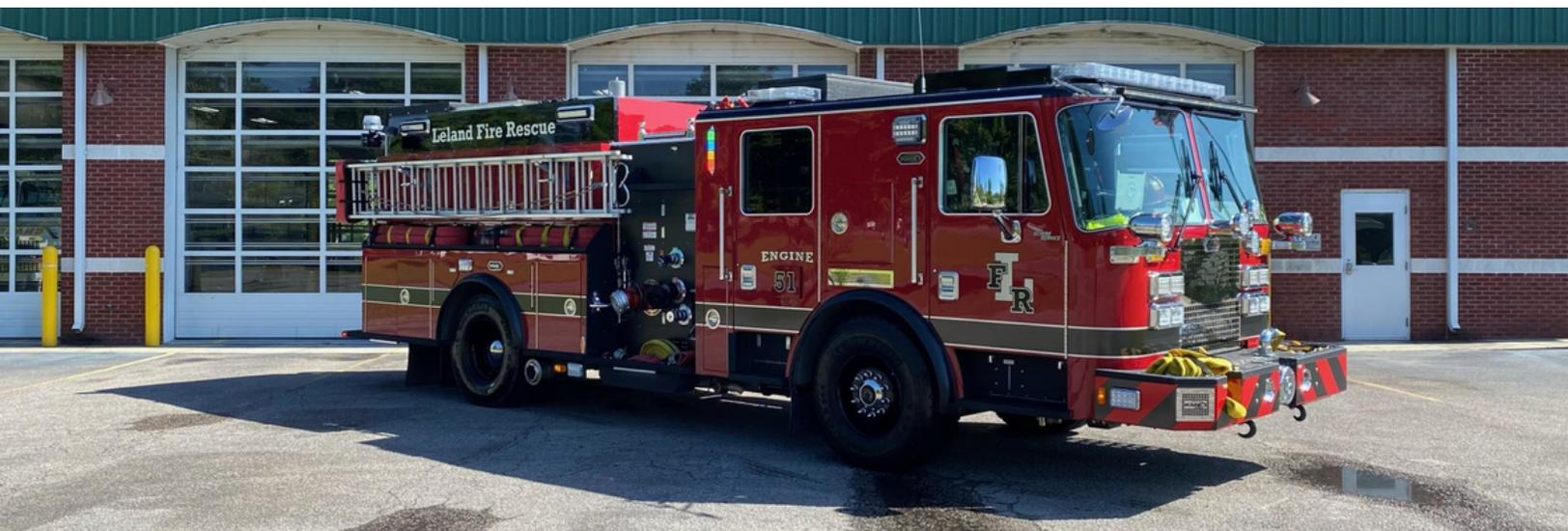
Engine 5171 is a 2022 KME Custom Pumper. Engine 5171 holds 750 gallons of water and has a 1500 gpm pump. It is housed at Station 51.
