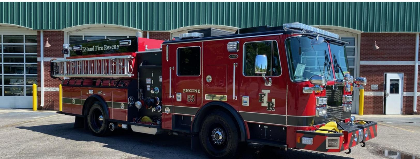
Engine 5271 is a 2022 KME Custom Pumper. Engine 5271 holds 750 gallons of water and has a 1500 gpm pump. It is housed at Station 52.
