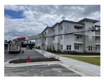
In this photo, the truck company is placed on the corner of a large multi family dwelling with aerial access to two sides. This is a good example for when the fire is on one end of a complex and maximum effectiveness of the aerial is utilized.
