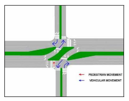
In Phase 1 of the crossing the pedestrian (or cyclist acting as a pedestrian) crosses the major street as the vehicles are turning left into and right out of the minor street.
