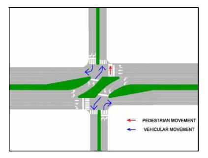
In Phase 3, much as in Phase 1, as vehicles are turning into and out of the minor street, pedestrians can cross the major movement.
