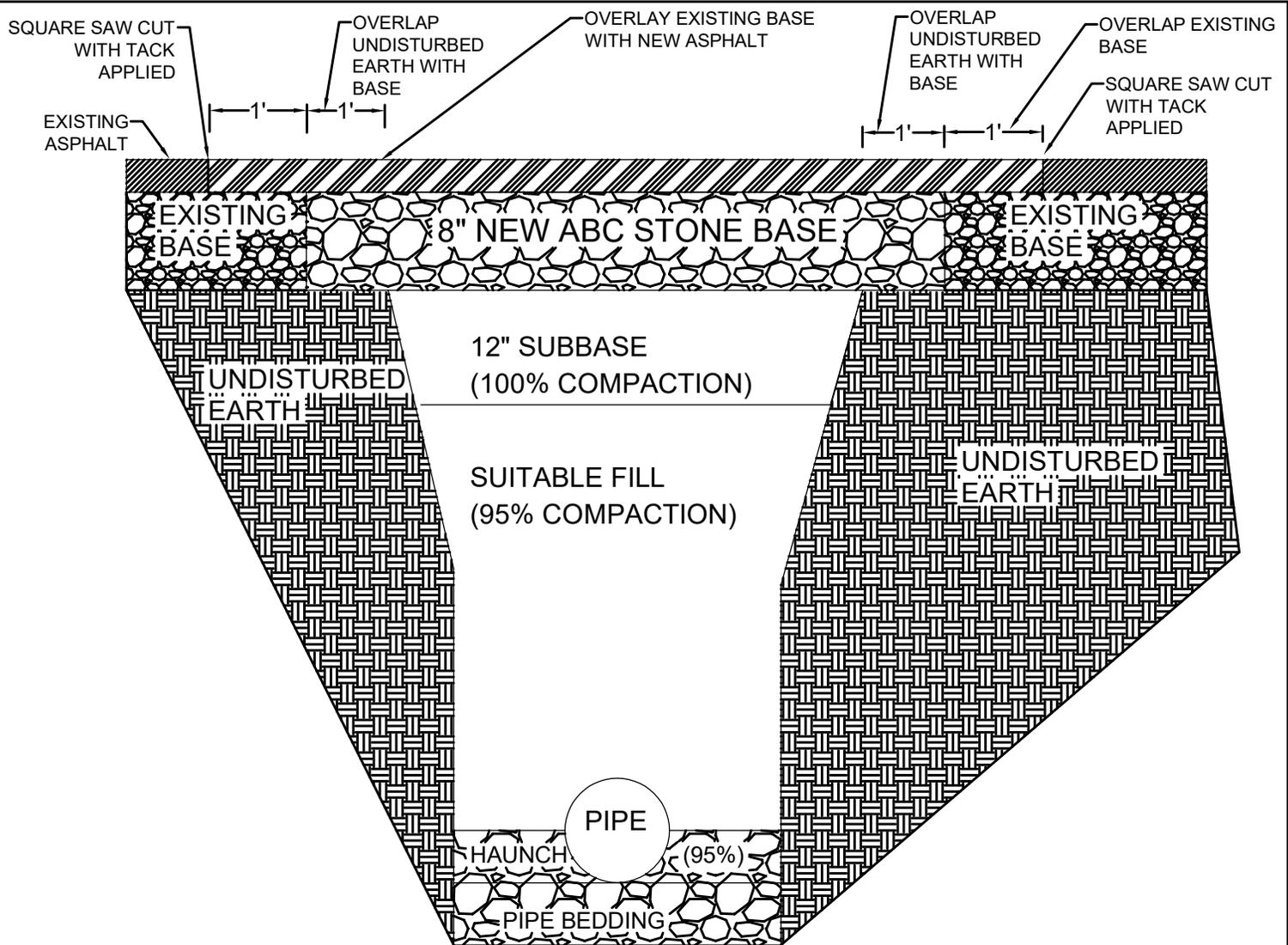
1. ASPHALT THICKNESS SHALL MATCH THE EXISTING ASPHALT THICKNESS OR BE 2" NC DOT S9.5B ASPHALT WHICHEVER IS GREATER.
